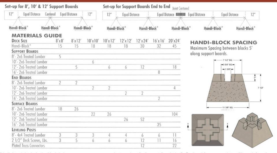
This lightweight deck pier block is in many ways a more convenient version of a "precast foundation". Produced from a proprietary fiber reinforced, cement-like material that is extremely lightweight. HANDI Block is designed to support an 1800 lb load and is setup to handle a 4x4 or 6x6 post with easy modification. Other benefits include:
